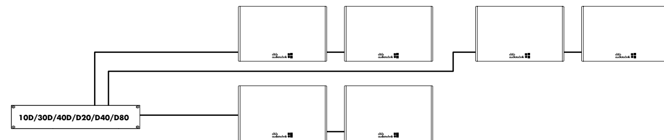
10D/30D/40D/D20/D40/D80 amplifier in mixed configuration with Dual Channel mode for MAX2, M6, M4 and 2-Way Active mode for M6 and M4
