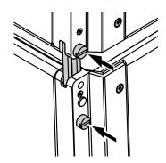
Fig. 4: SUB to SUB, 2° splay, blocked
