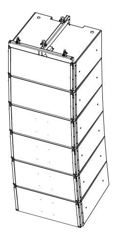
**KSLi-SUB colum, 6-deep, 2° splay with:** Z5744 KSLi-SUB Mounting frame
