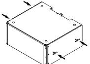
2. Attach the T-handles and position the cabinet below the frame.
