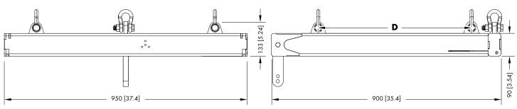
**Z5744 KSLi-SUB Mounting frame dimensions in mm [inch]**
