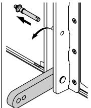
Splay/Rear link mechanism
