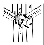
Fig. 3: SUB to SUB,  $2^{\circ}$  splay, free
