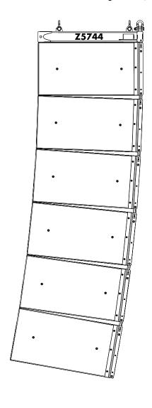
**KSLi-SUB column, 6-deep, 2° splay with:** Z5744 KSLi-SUB Mounting frame
