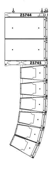
**Mixed array with:** Z5744 KSLi-SUB Mounting frame Z5745 KSLi-SUB Mounting adapter
