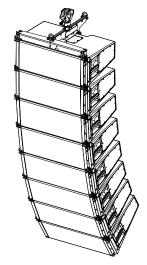
XSL8/12 Line array 8-deep Tension mode - Front, Mounting frame with Rota clamp
