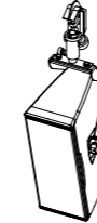
T10 point source or Ti10P with Z5371 T Flying bracket Z5010 TV Spigot with fixing plate Z5012 Pipe clamp for TV Spigot
